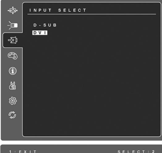
The screenshot shows the 'INPUT SELECT' menu. On the left is a vertical toolbar with icons for brightness, contrast, input select, information, and settings. The 'INPUT SELECT' menu itself has a header 'INPUT SELECT' and two options: 'D - S U B' and 'D V I'. The 'D - S U B' option is highlighted with a white border. At the bottom of the menu are two buttons: '1 : EXIT' on the left and 'SELECT : 2' on the right.
